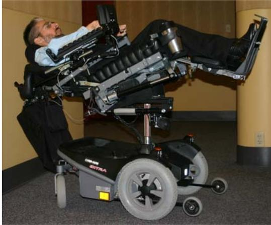
Fig. 11: Seating System Fully Reclined
