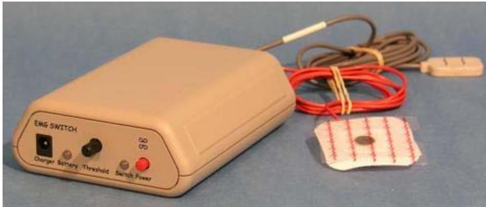
**Fig. 1:** Tinkertron Dual D-Box, Delsys EMG Sensor, Reference Electrode, and Stickers
